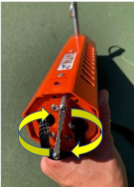
**Exhibit D:** Push handle in and rotate clockwise to increase resistance. You will hear a “click” when mechanism is locked into place. We recommend starting slightly less than one revolution for sprint work.
