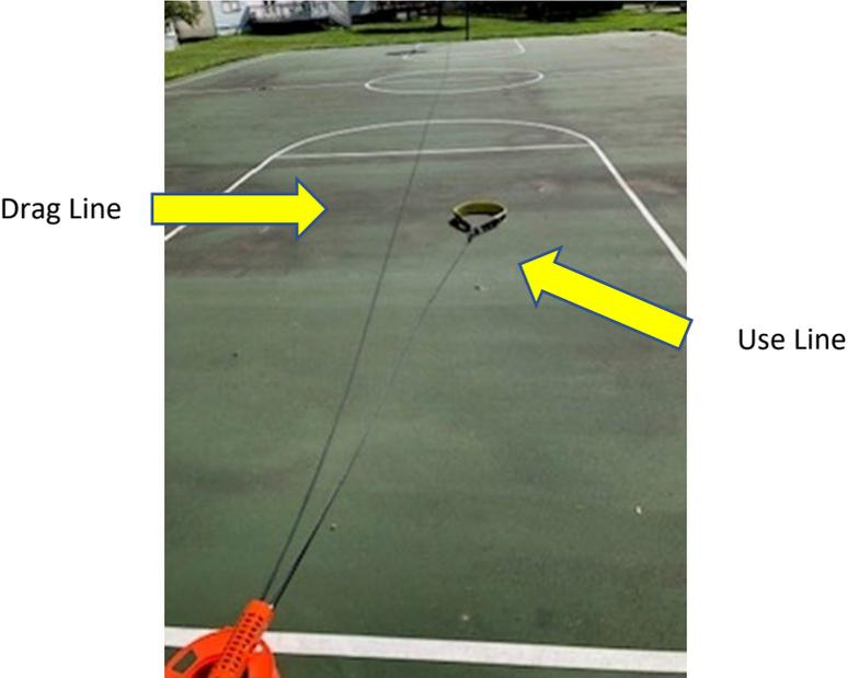
**Third**, make sure the drag line is kept stretched out do not coil it near the machine on the ground. The coil can lead to inconsistent resistance as the rope struggles to unwind and increases the likelihood of knots and snags (see **Exhibit G**).
