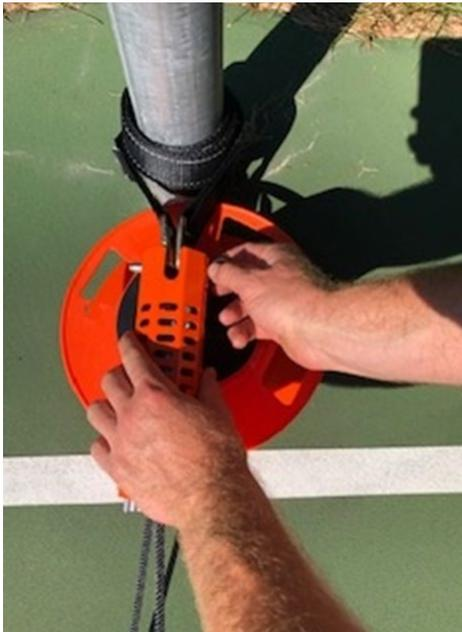
**Exhibit H** : Picture on the left shows incorrect grip on pin, and picture on the right shows correct use of key ring to pull out pin.
